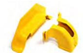
TC1279-89KIT Side drop-off to 50mm (2") square convoluted tube (TC1279 - 85YEL) • Can fit approx. 100-150 x 2mm cables • Also includes duct ramp
